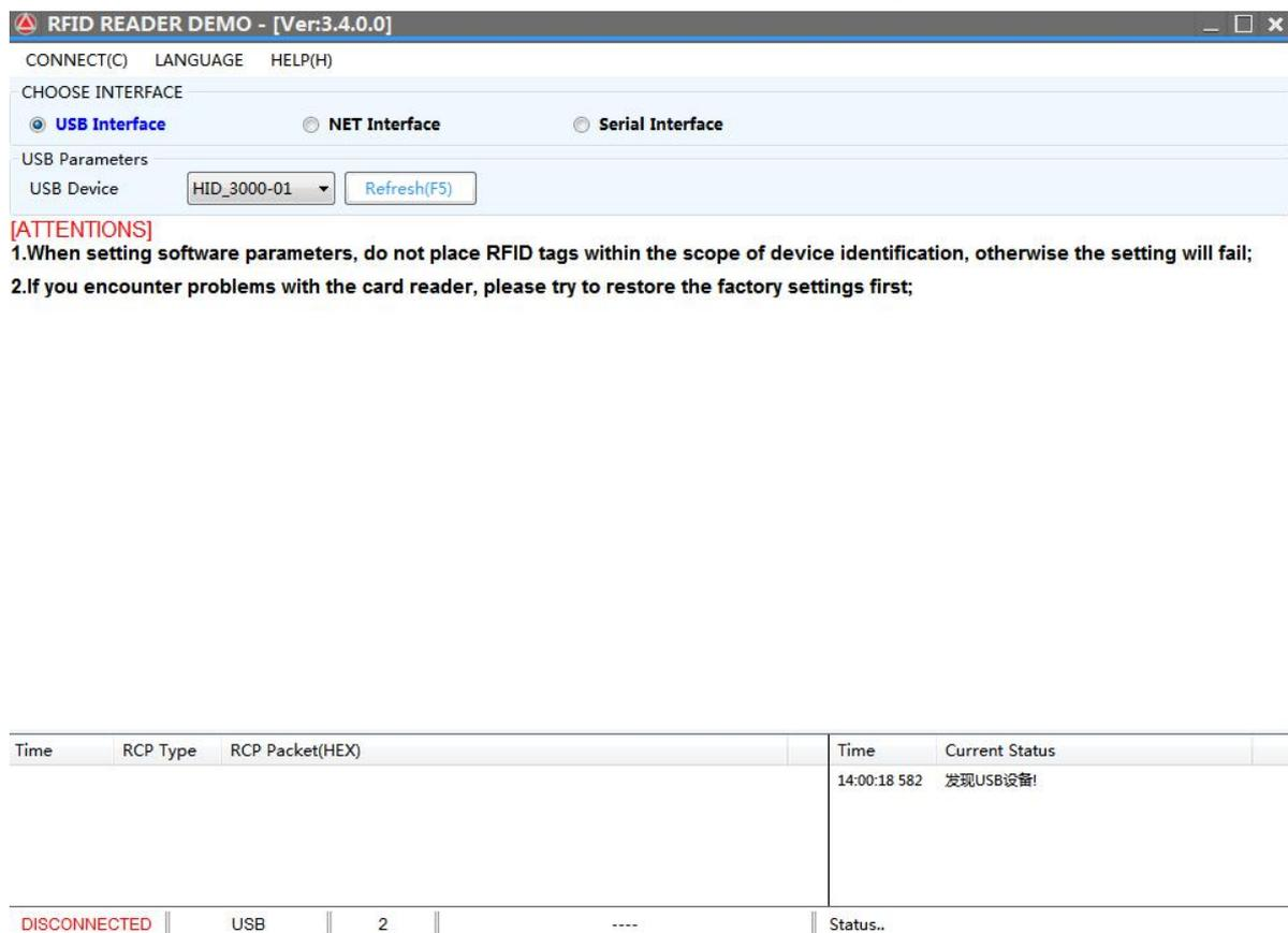
There are three communication parameter configurations: USB Interface---serial Interface---net Interface. The parameter configuration of each interface is different, so you can connect to the computer only by choosing the correct configuration.
