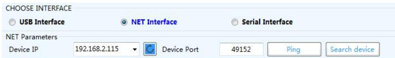
Here, select the correct remote IP address and remote IP port of the equipment (by default, the computer is the customer service terminal, this equipment is the server, and TCP/IP protocol), and click the "Network Diagnosis" button. If the connection is correct, the success sign will be displayed in the status bar, as shown in the figure:
