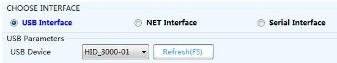
If the USB device is empty, please confirm whether the usb cable is plugged in again, and then press the button  or F5.
