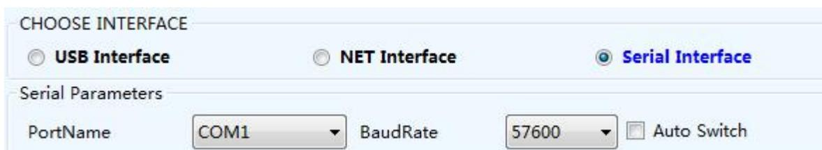
Select the serial port that appeared when the converter was installed before, the baud rate is 57600 by default, and click the "CONNECT" button.
